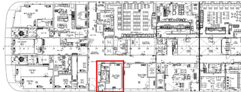
Figure 55 - Plan view of the Deck A of the cruise ship, showing the location of the space to be refitted for SSE equipment installation
