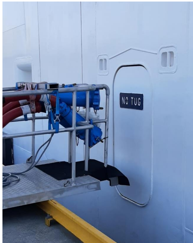
Figure 56: Outside view of the Cruise Case study vessel highlighting SSE cables entrance
